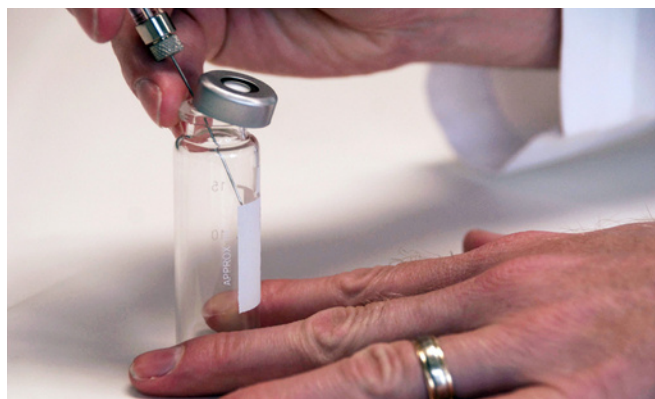
Figure 1. Introducing an eau de cologne sample into a HS vial.
